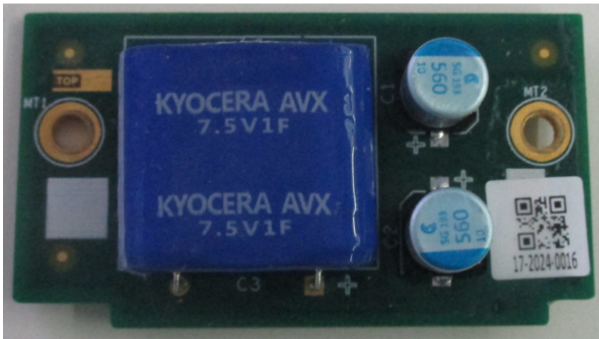
EUT – Top View of Super Capacitor PWB
